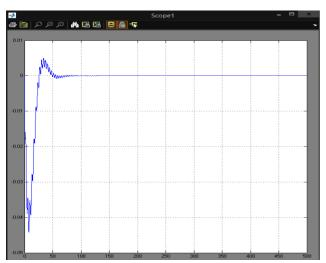
Figure 5 Frequency Deviation of Double Area System with PSO based PID controller of Area- 2
