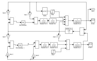
Fig. 2: Purposed Model of Two Interconnected Area ALFC
