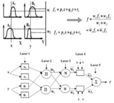
Fig.3. Schematic of fuzzy and neurofuzzy paradigm: (a) Fuzzy inference system and (b) equivalent Neurofuzzy architecture.
