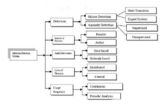
Fig. 2: Classification of IDS based on its characteristics
