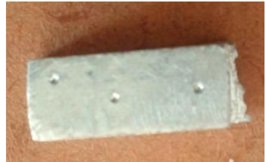
Fig-8 MMC specimen after Hardness test
