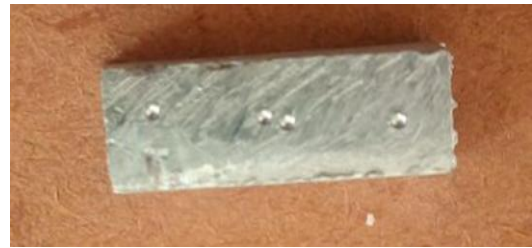
Fig-7 Sand casting specimen after Hardness test.
