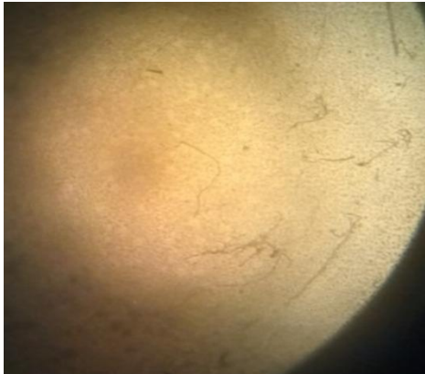
Fig -6. Microstructure of sand casting specimen
