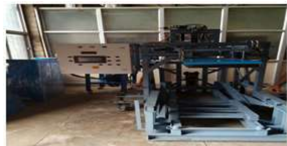
Figure 2: Rolling Compactor cum Rut Analyser
