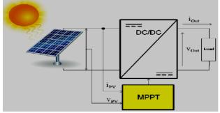
Figure 1: Module and dc/ dc converter with MPPT
