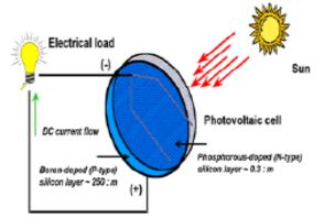
Figure 2: Working of Photovoltaic cell
