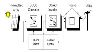
Figure 3: Structure of PV Power System
