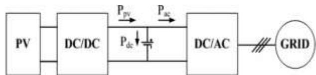
Figure 5 Simplified block diagram of two-stage MIC
