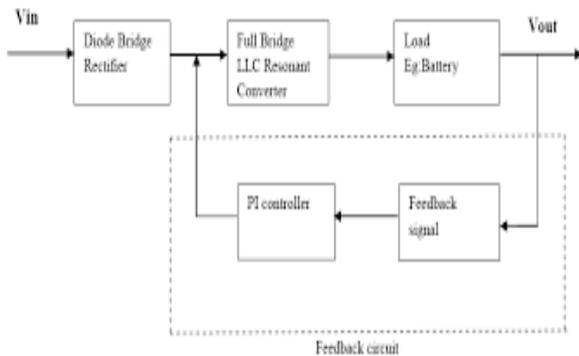
Figure 2 Block Diagram of Full Bridge LLC Resonant Converter for Battery Charging Application.
