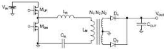
Figure 4 Scheme of a single module LLC resonant converter.
