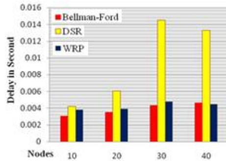
Figure 2 Delays vs. Number of Nodes
