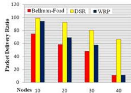
Figure 3 Packet Delivery Ratios vs. Number of Nodes
