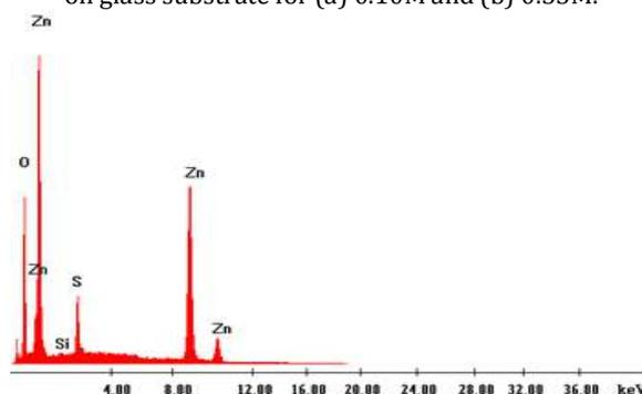
Figure 3 EDAX spectrum of ZnS thin film of 0.3 M.
