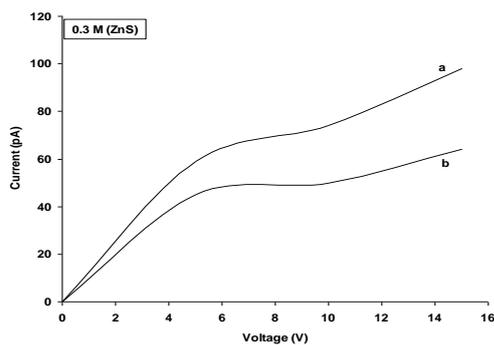
Figure 6 I-V characteristic curve of ZnS thin film (0.30M) (a) Current under illumination (b) Dark current.
