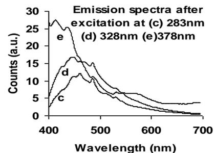
Figure 9 Excitation and emission spectra of nanocrystalline ZnS thin films a - emission at 448 nm, b - emission at 486 nm, c - excited at 283nm d - excited at 328 nm, e - excited at 378 nm
