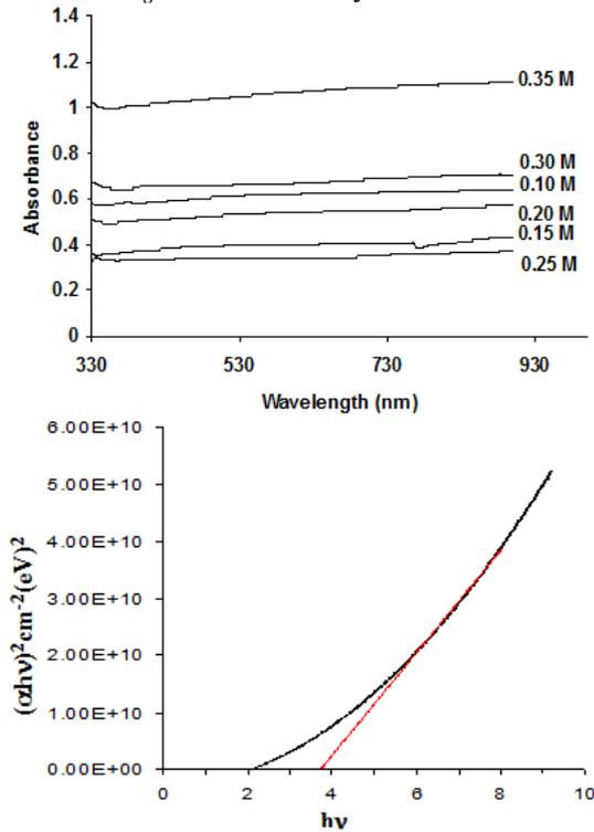
Figure 5 Plot of  $h\nu \sim (\alpha h\nu)^2$  of ZnS thin film on glass substrate at room temperature.
