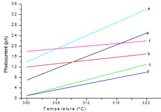
Figure 6 Characteristic curve of Temperature vs Photocurrent of ZnS thin films (a – e correspond to 0.10 – 0.35 M).
