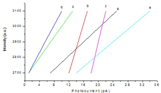
Figure 7 Characteristic curve of Photocurrent vs Illumination of ZnS thin films (a – e correspond to 0.10 – 0.35 M).
