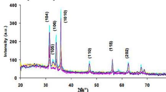
Figure 1 XRD pattern of ZnS prepared by CBD on glass substrate for different molarities (0.10, 0.15, 0.20, 0.25, 0.30 & 0.35 M).
