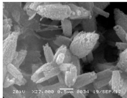
Figure 2 SEM micrograph of PVA capped ZnS nanocrystals on glass substrate for (a) 0.10M and (b) 0.35M.
