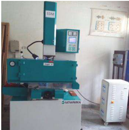
Fig.2. Photographic view of ZNC 5030 die-sinking EDM
