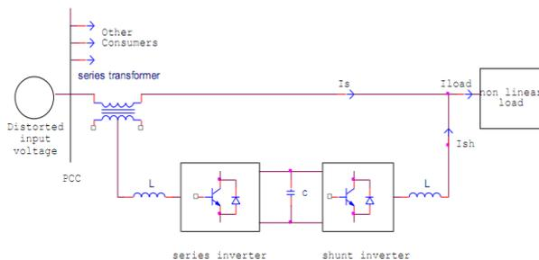
Figure 1 Basic block diagram of UPQC
