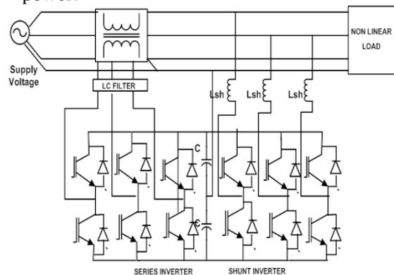
Figure3: Three-phase four-wire UPQC
