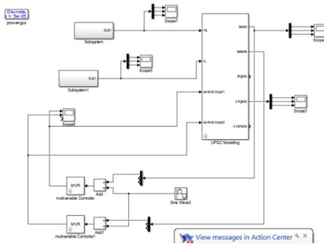
Figure 9: Simulink model of UPQC
