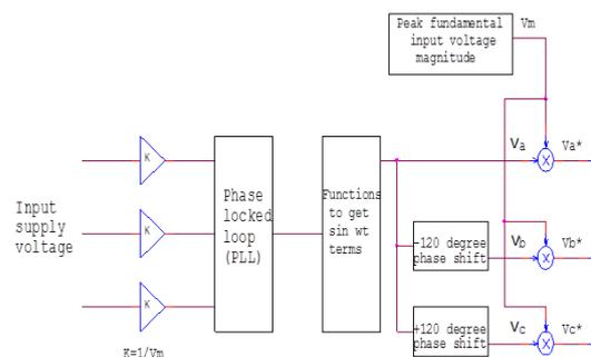
Figure.7: Generation of Unit Vector Templates and reference Load Voltages
