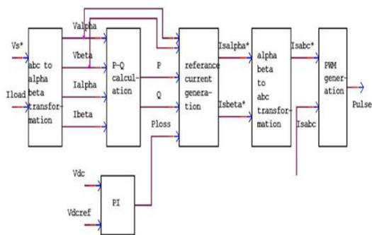
Figure 9: Control algorithm of PAF
