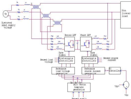
Figure 8: Overall Control Circuit
