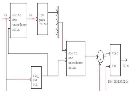
Figure 8: Control algorithm of SAF
