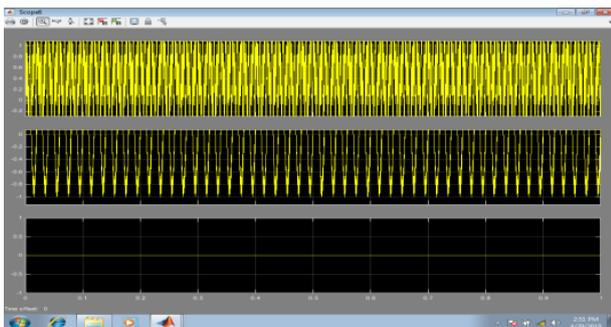
Figure 11: Multilevel Converter Output
