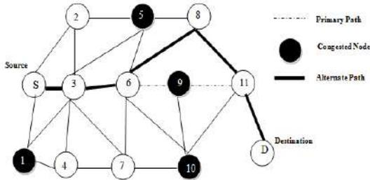
Figure 3 Alternate path finding process in CFR
