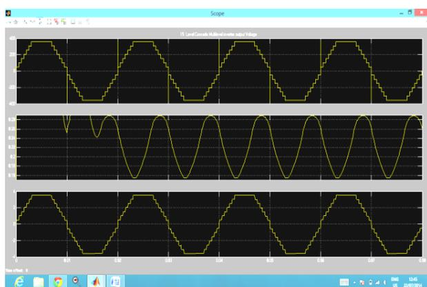
Figure10: 15 level waveform of solar inverter
