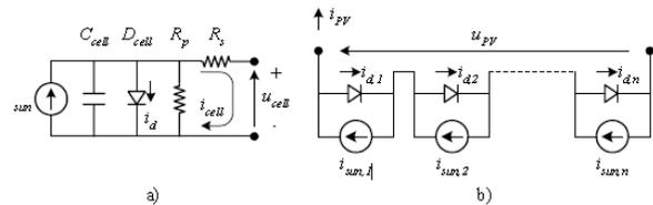
Figure 3: Electrical model of a PV cell (a) and of a PV module made up around n cells (b).
