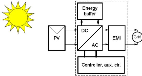
Figure 4: Block-diagram of an inverter for PV system.
