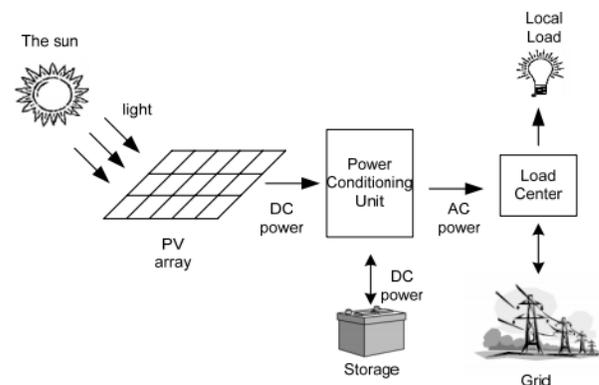
Figure 1: Components of grid connected photovoltaic system.
