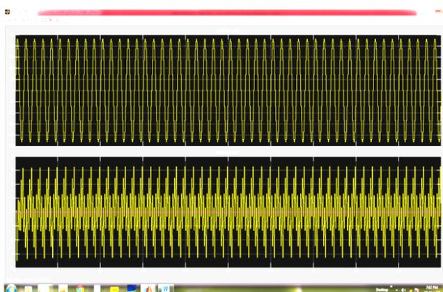
Figure11: 11 level waveform which injected in grid
