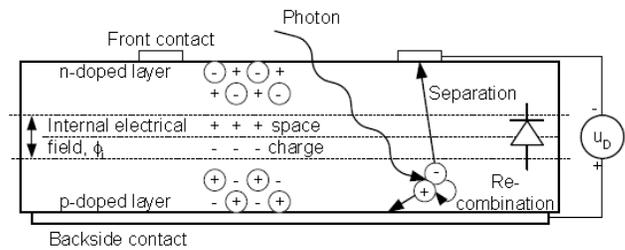
Figure 2: Cross section of an abrupt PN junction
