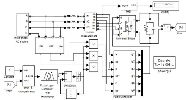
Figure 7 Simulated power circuit for Fuzzy controlled improved power quality converter
