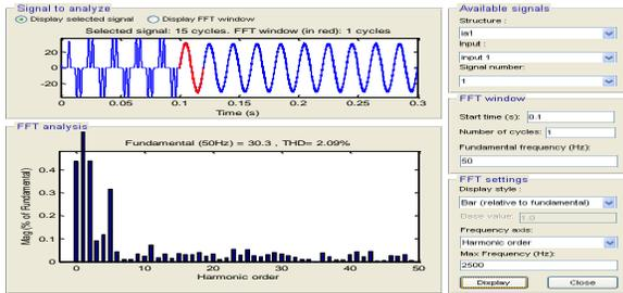
Figure 10 Harmonics spectrum with PI controller
