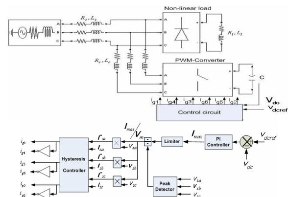
Figure 2 (a) Active filter system, (b) Active filter system using PI controller
