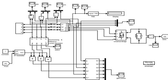
Figure 5 Simulated power circuits without controlled improved power quality converter
