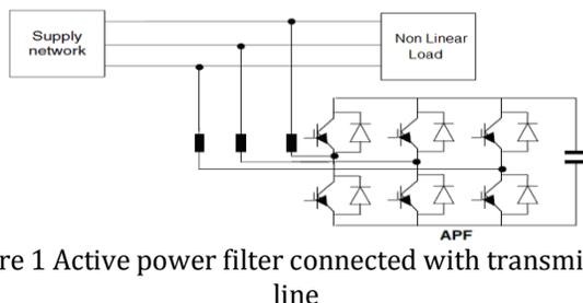
Figure 1 Active power filter connected with transmission line
