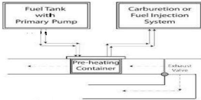
**Figure 1 preheating setup**
