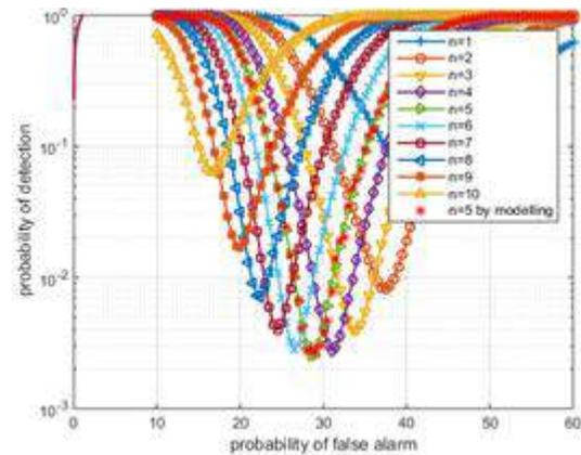
Figure 5: Probability of detection Vs Probability of false alarm at 10dB SNR
