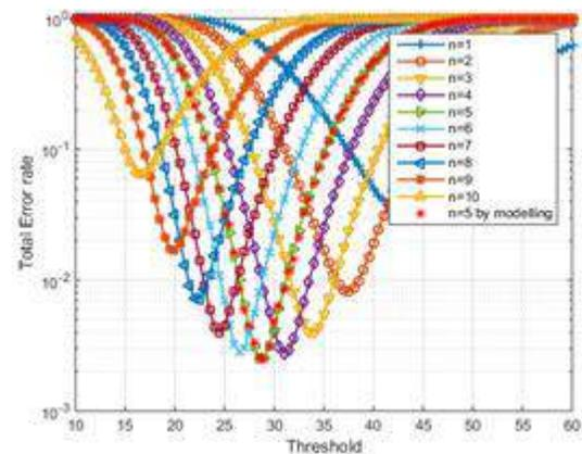
Figure 6: Threshold Vs Probability of total error rate at - 10dB SNR
