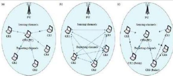
Figure 1: Classification of cooperative sensing (a) Centralized (b) Distributed (c) relay-assisted.
