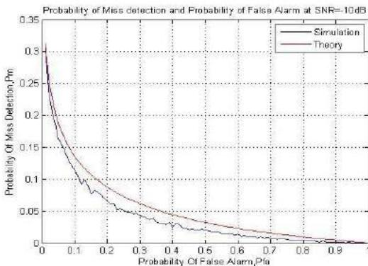
Figure 8:  $P_m$  vs.  $P_{fa}$  at SNR=-10dB
