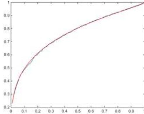
Figure 9: Probability of Detection vs. SNR (dB) at  $P_{fa}=0.4$ .
