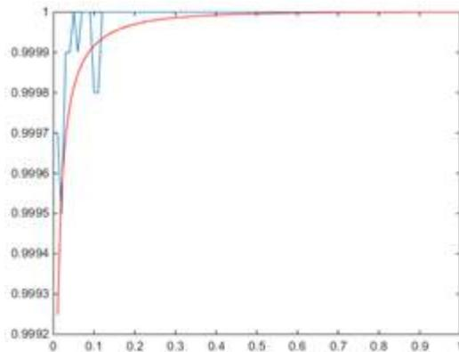
Figure 7: Probability of Detection vs. SNR (dB) at  $P_{fa}=0.2$  for channel
