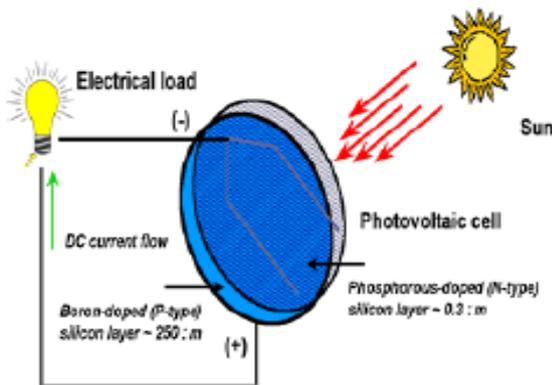
Figure 2: Working of Photovoltaic cell
