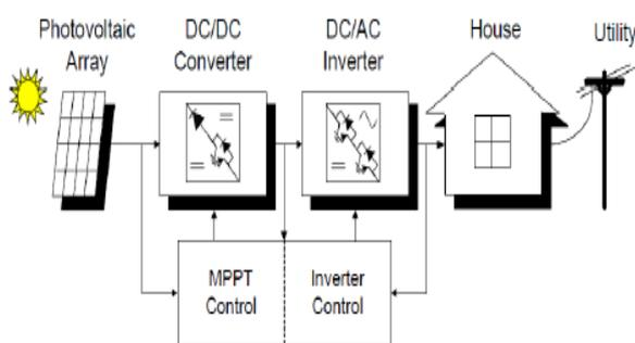
Figure 3: Structure of PV Power System
