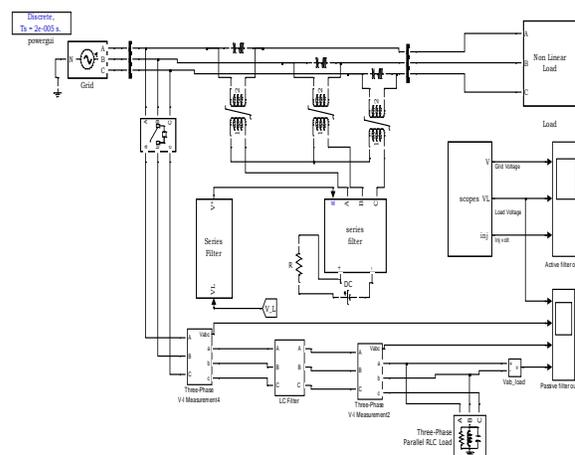
Fig.1. Simulink model of THD analysis for the improvement of power quality in three phase AC system by using active passive filter
